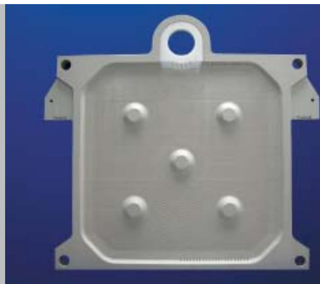
Combination chamber plate 2000 x 2000 mm with maximum chamber volume for high throughput. Abrasion protection at the slurry feed hole.
