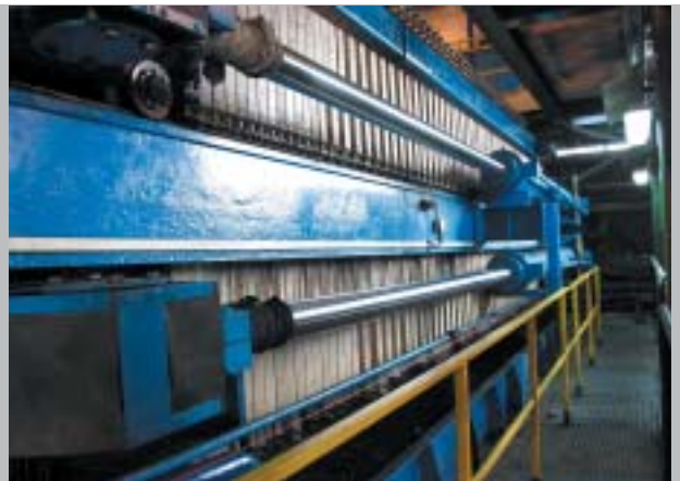
SALA filter press with JVK membrane- and combination chamber plates 1500 x 1500 mm
