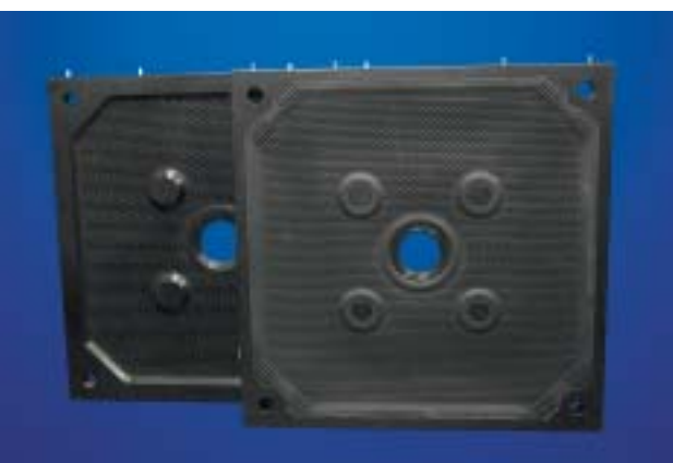
Membrane- and combination chamber plate 1200 x 1200 mm. PVDF plate and EPDM membrane are electric dischargeable. Application at extremely high temperatures and/or with aggressive chemicals.
